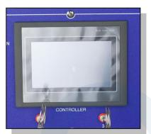
Touch-screen model, to set the parameter of testing
