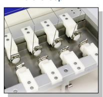
4 group of fixture; Fixed the sample our the cylinder, one this the fixed fixture, the other one the movable fixture.
