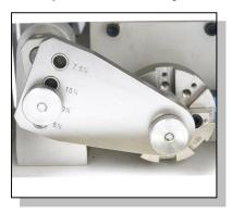
Adjust the displacement of flexing.
